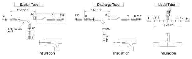
\*Insulators for both the Suction tube and the Discharge tube are the same.
